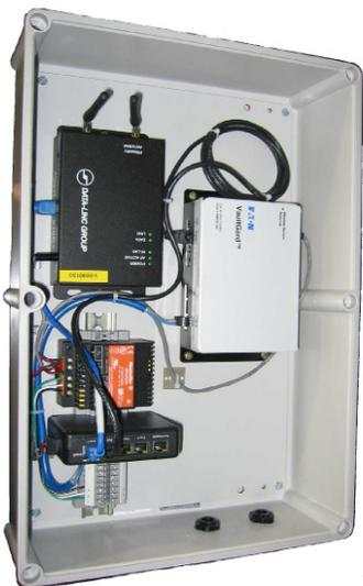
The standard VaultGard is provided in a NEMA-4X (IP66) rugged Wall-mount enclosure.
